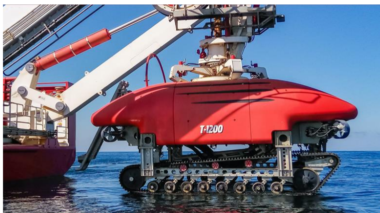
Figure 12: Example Jetting/Trenching Unit
