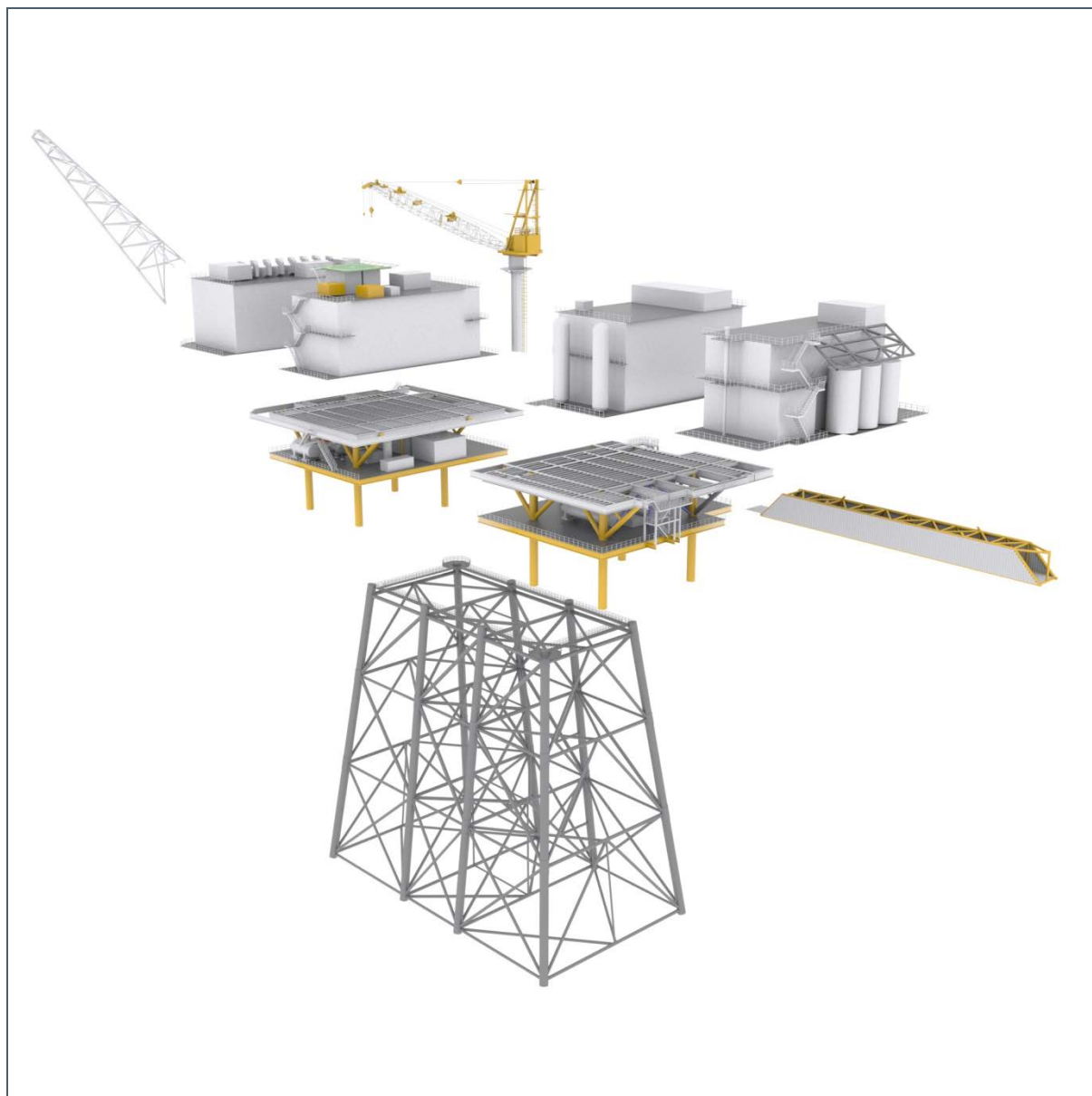
Figure 2.5 – Beatrice AP Schematic showing Exploded View of Topsides Modules
