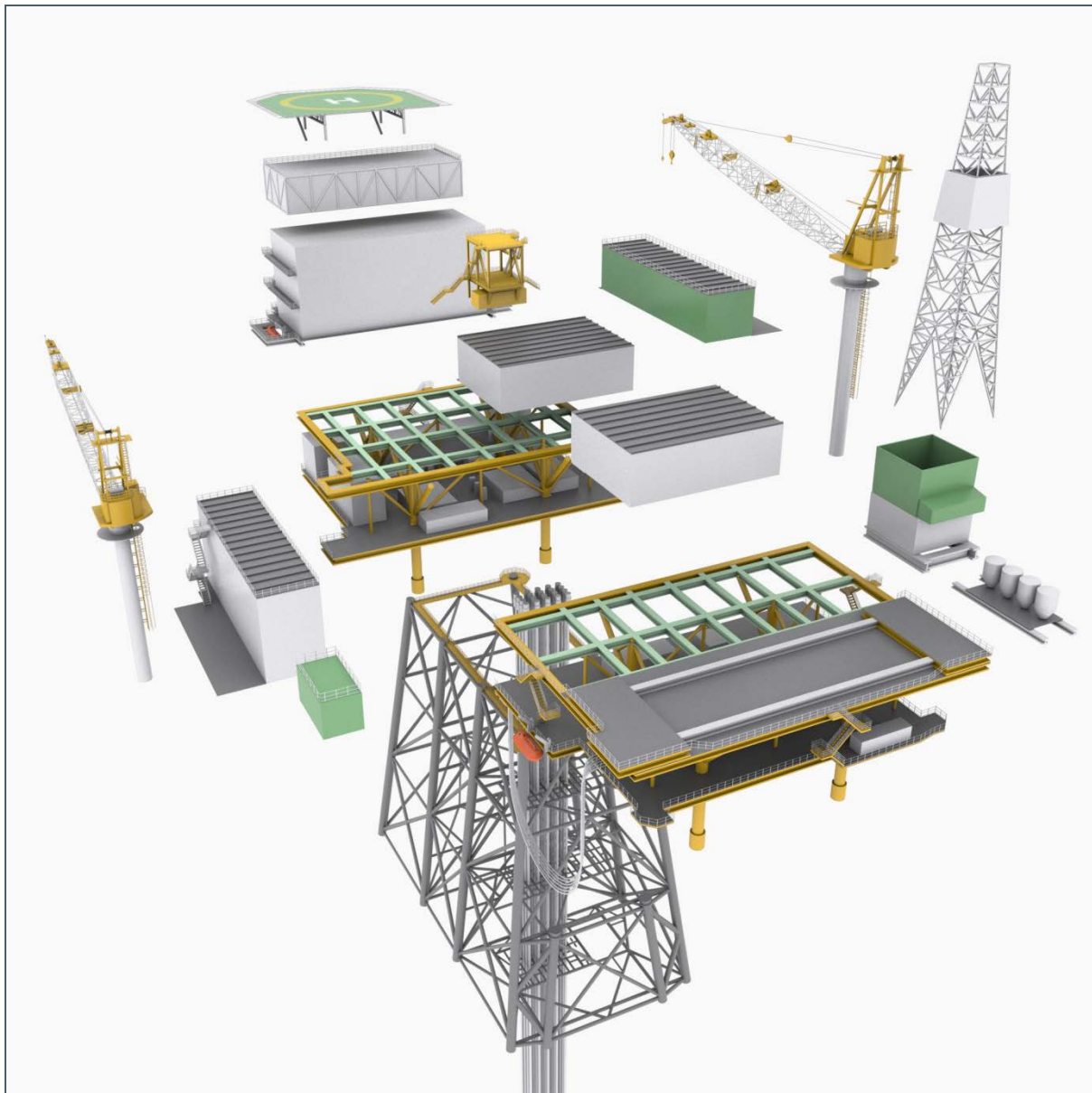
Figure 2.4 – Beatrice AD Schematic Showing Exploded View of Topsides Modules
