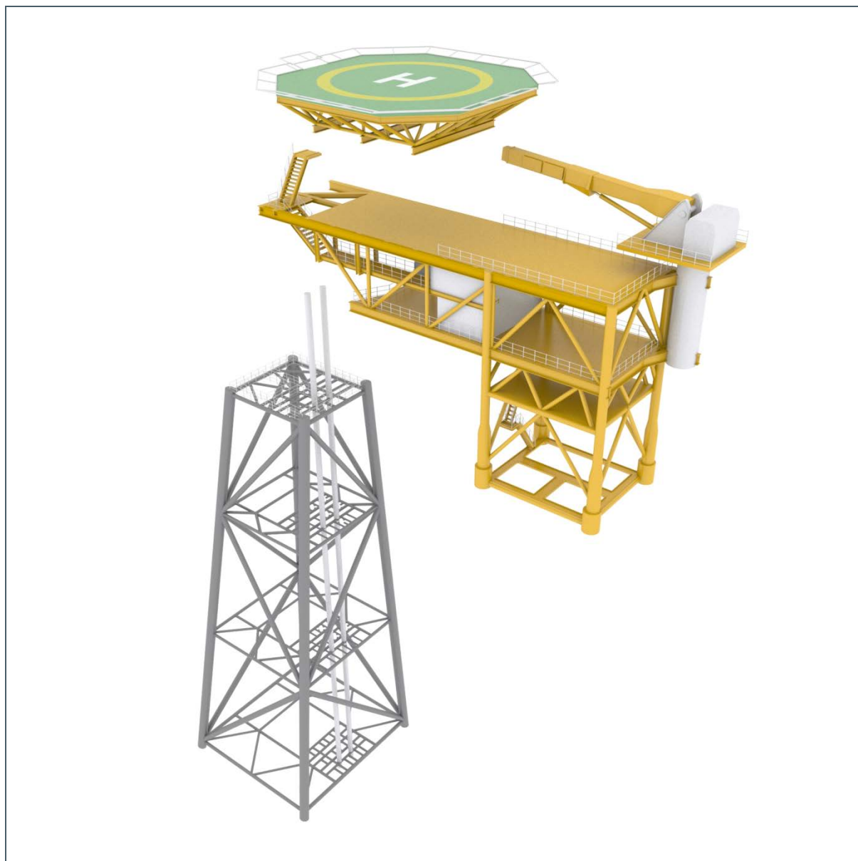
Figure 2.7 – Beatrice C Schematic Showing Exploded View of Topsides Modules
